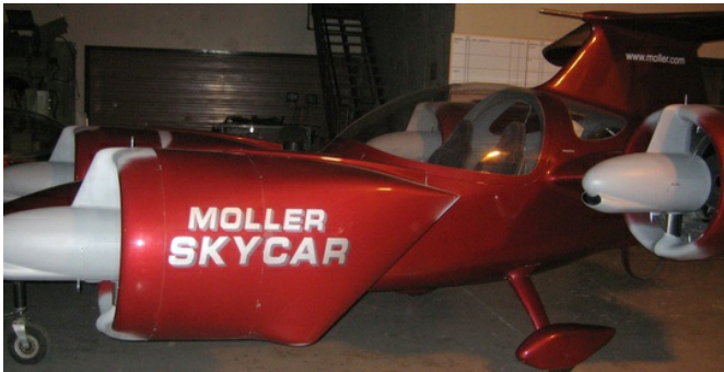
Photo: Side view of the M400 Skycar from Moller Int. Personal aircraft vehicle capable of vertical liftoff, landing, hovering and cruising. Credit: Me! (aka Erin Richards)
